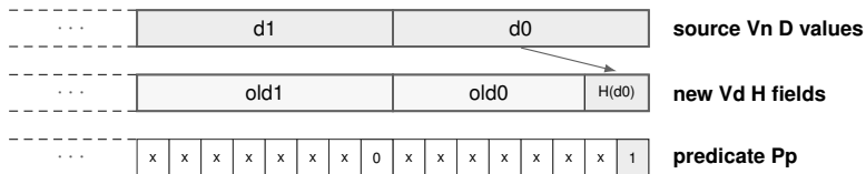
VFCVTH.D double-to-half conversion containers
